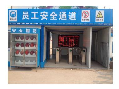
With ZKBioSecurity 3.0 software and tripod turnstile hardware, ZKBioSecurity smart construction site entrance control solution can effectively control the access information of the construction site and display the verify information on LED screen.
